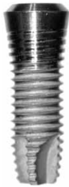
Fig. 10. Partially grooved flange of 3i TG 2410 implant.
