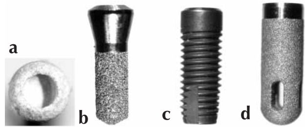
Fig. 7. (a) Apical chamber in Minimatic IHCSHA315. (b) V-shaped apex in Tenax 10-S. (c) Flat apex in Astra Fixture 4.0. (d) Curved apex in Integral 0802.
